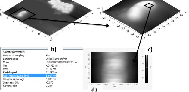
Figure 1. AFM of cells of bacteria of genus *Lactobacillus*. a) 2-dimensional image of group of cells and lateral profile of section; b) 3-dimensional image of group of cells and single cell; c) the enlarged 3-dimensional image of single cells; d) parameters of level of a roughness (RMS) of a site of a single cell.
